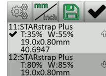
☞ With the OK key you can, without saving the changed setting, activate the active dataset with the original setting or activate a different data set.
